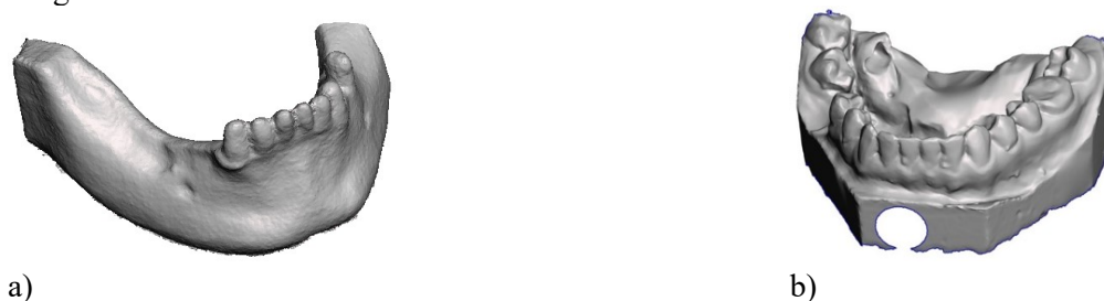
Fig. 4. 3D models obtained using a) close-range photogrammetry and b) structured light 3D scanner
