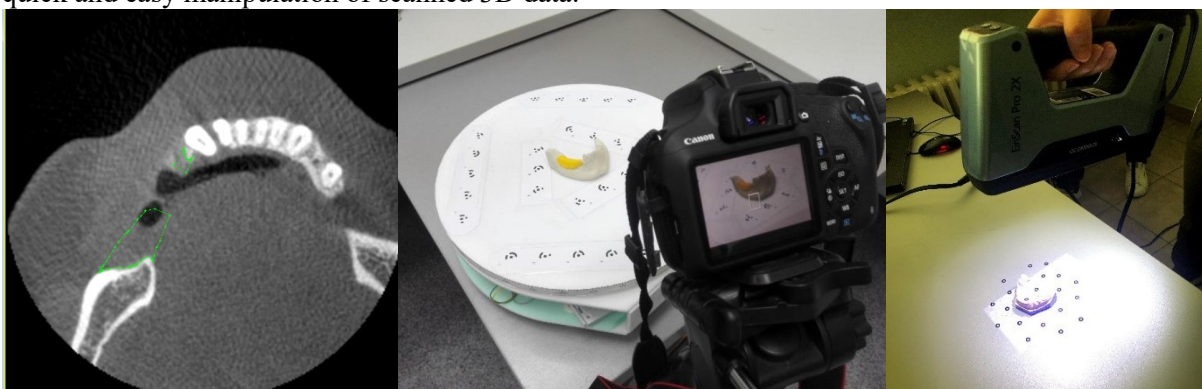
a) b) c) Fig. 2. 3D digitization of physical models using a) CT scanner, b) close-range photogrammetry [10] and c) structured light 3D scanner
